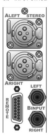
The **A Stereo Input** is via standard female XLR-3 connectors and it is set for **LINE** sources. The input is electronically balanced and it is factory-preset for a 0 dB level (ref to § 8.8 for Sensibility adjustement).
