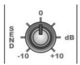
It adjusts in the +/- 10 dB range the level of *mix-minus* signal which is sent to the telephone caller via the external telephone hybrid.
