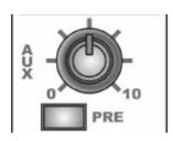
This control sends the input channel signal to the Auxiliary bus (range - $\infty$  to 0 dB max). As AUX bus is separated from the main outputs, it can provide additional output for foldback, echo units or extra loudspeaker feed.
