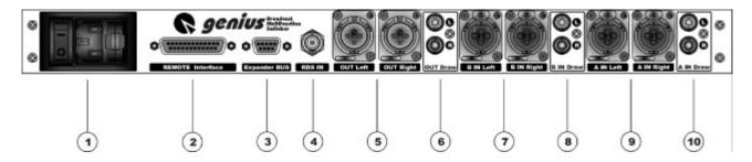
① **ON/OFF switch:** it switches on the equipment, the led inside shows the status of the equipment. If the led is off and the switch is ON please check the power supply wire and the PWS protection fuse integrity
